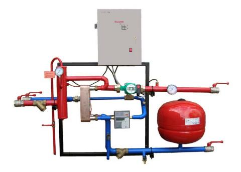
Compact heat substations are available as small (RTP) and medium sized (KTP) with heat capacity from 20kW up to 500 kW. They are small, lightweight, with compact construction and easy to install in small and narrow spaces.
